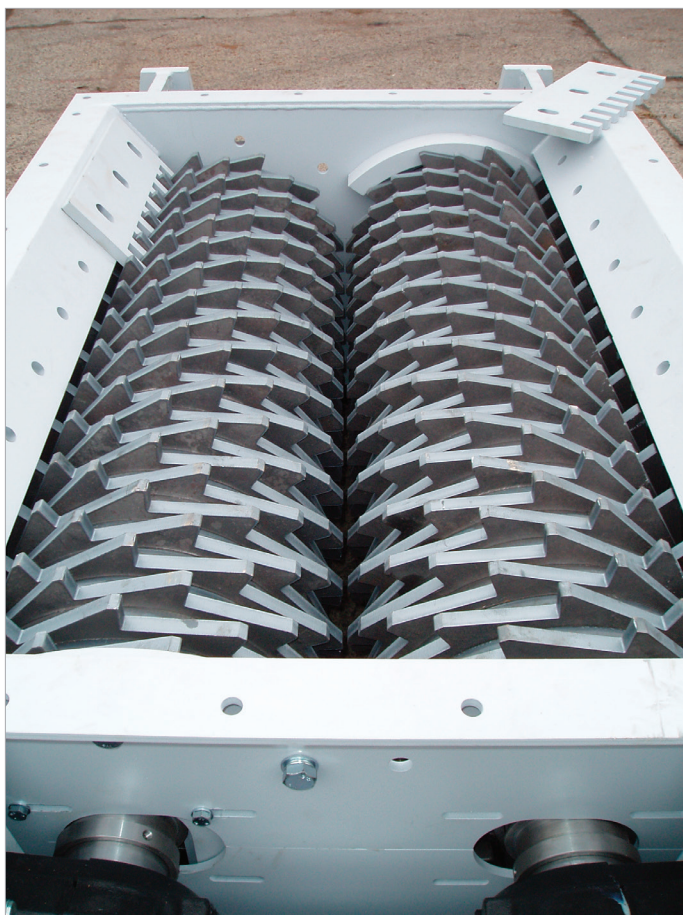
Obr. 2: Drtič strusky DS-500.
