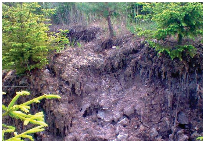
Fig. 10: Tension crack on the southern slope of Lake Medard below the village of Bukovany in 2017.
