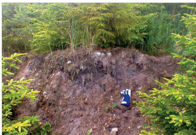
Fig. 12: Tension crack on the southern slope of Lake Medard below the village of Bukovany in 2019.
