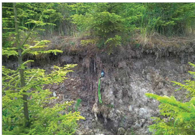
Fig. 11: Tension crack on the southern slope of Lake Medard below the village of Bukovany in 2018.
